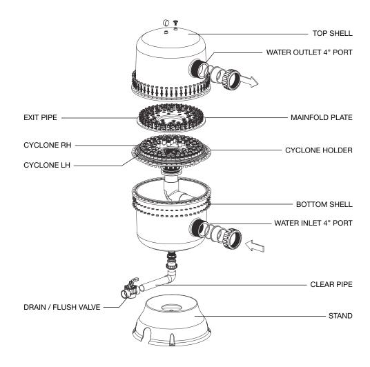
Incoming water is guided by a diverter plate so that it enters multiple hydro cyclones tangentially generating a strong centrifugal effect. This spins the sediment out to the hydro cyclone's wall and then spirals it down to the sediment chamber, while the cleansed water spirals upwards.
