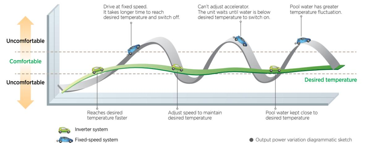
Electroheat ECO-V inverter pool heat pumps utilise a variable speed compressor to regulate the pool water temperature automatically and independently.
