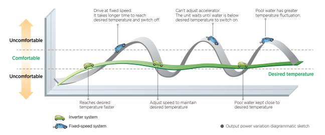
Electroheat ECO-V inverter pool heat pumps utilise a variable speed compressor to regulate the pool water temperature automatically and independently.
