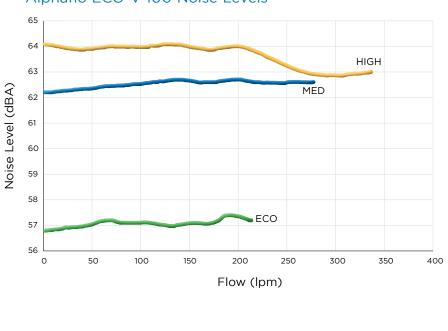
ECO speed (1900rpm)Medium speed (2410rpm)High speed (2850rpm)
