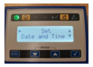
Once in the setting, change the date and time to the current Australian Eastern Standard Time (AEST). To scroll through the setting in each menu use the tick button ( ) to scroll right and the ESC button ( ) to scroll left. Use the up and down button to change the setting values. When completing any changes in the menu always click the tick button to get to the end of the changes to save the settings.
