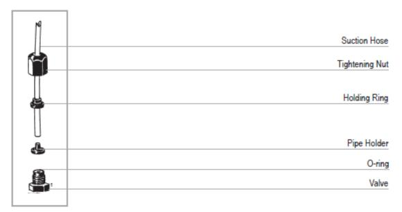
Figure 5.11 Connection Point Assembly6
