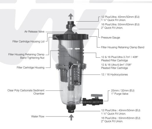
**Note:** The MultiCyclone Plus/Ultra centrifugal section is designed to filter sediment that is heavier than water; floating debris cannot be filtered out by centrifugal filtration.
