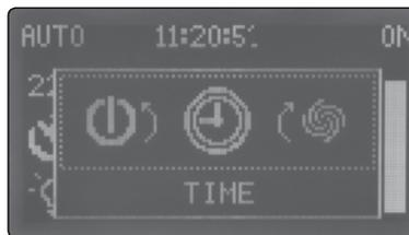
Electrochlor has a digital clock and 4 independent timers. Each of the timers can be programmed independently to have different behaviour and control different devices (outputs).
