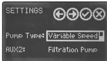
**Note:** The control of the variable speed pump is executed via communication cable. When the pump is controlled via the communication cable the pump can be connected to an independent power output. This enables the pump GPO to be used as an independent output to control a secondary pump (booster pump) or any other equipment that needs to be operated at the same time of the pool pump. This also can be used to interlock functions. Please refer to the Interlock section below for more information.
