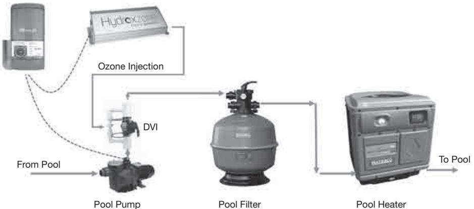
**1.1 Typical Installation of Hydroxzone**
