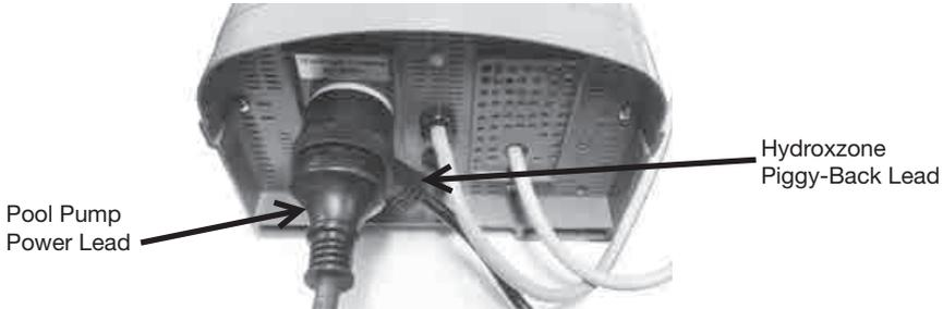
Connection of the Hydroxzone unit to a salt water chlorinator.
