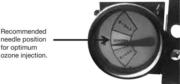
**Figure 2.8 Pressure differential indicator**
