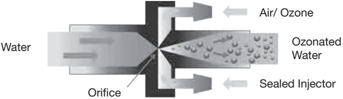
Figure 1.2 How the injector works
