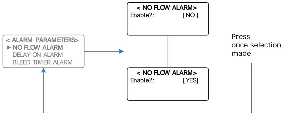
If the No Flow Alarm is enabled, the Alarm will activate when there is no flow detected by the optional flow switch.
