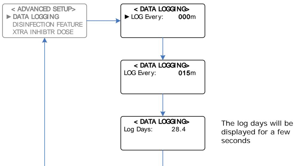
**Example:** Increasing Data Logging times from 0min to Log every 15min
