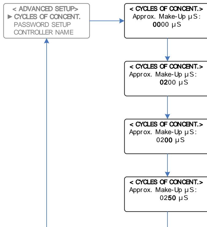
**Example:** Entering a Make Up Water Conductivity of 250  $\mu$ S
