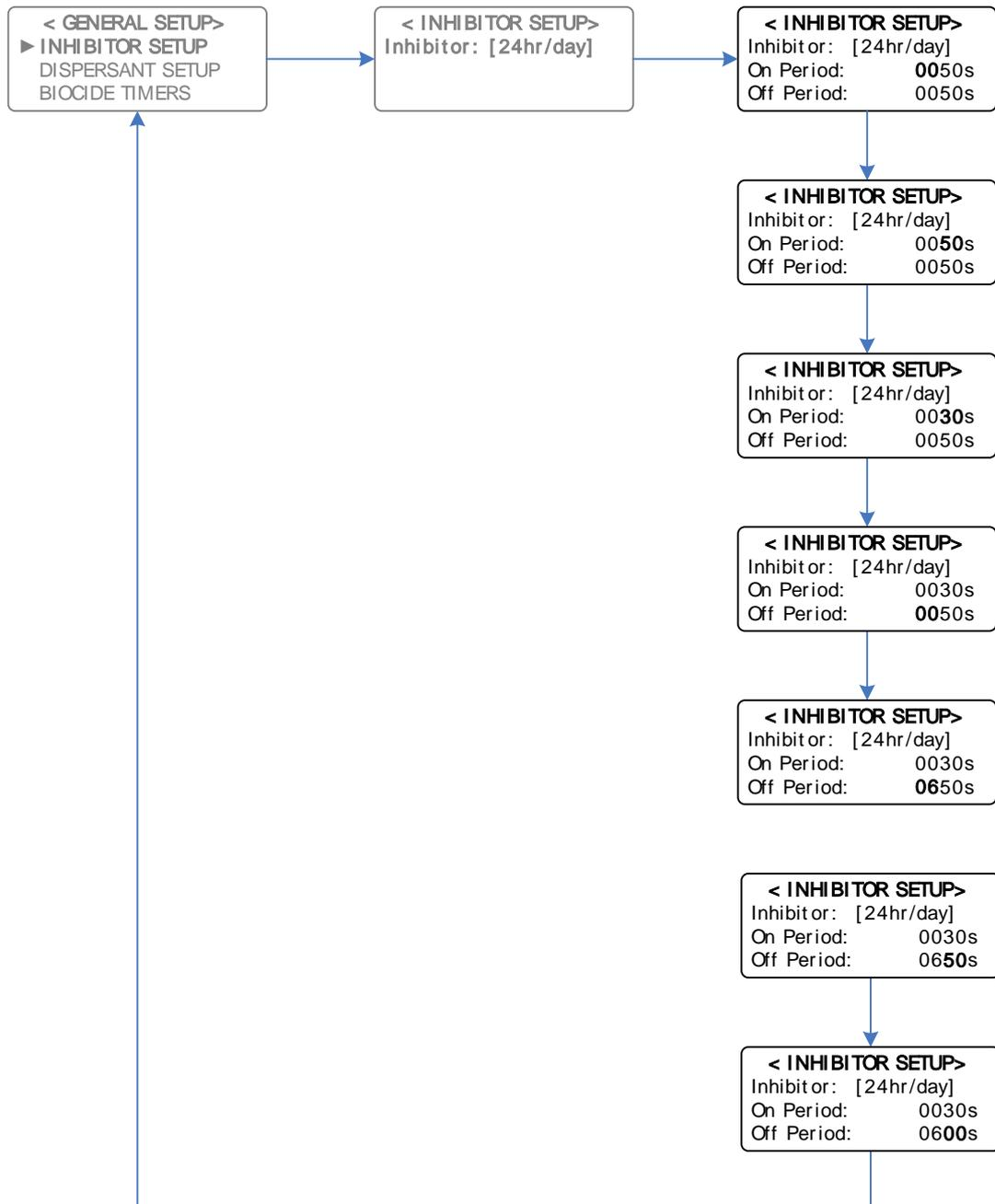
**Example:** With Inhibitor on "24hr/day" mode currently set – Setting the Inhibitor pump to repeat dose for 30 seconds followed by a 600 second off period
