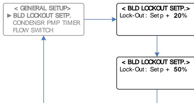
**Example:** Increasing Lockout Setpoint from Setpoint +20% to Setpoint +50%
