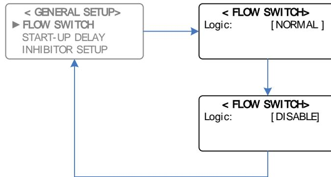
**Example:** Disabling Flow Switch Operation from Normal Logic
