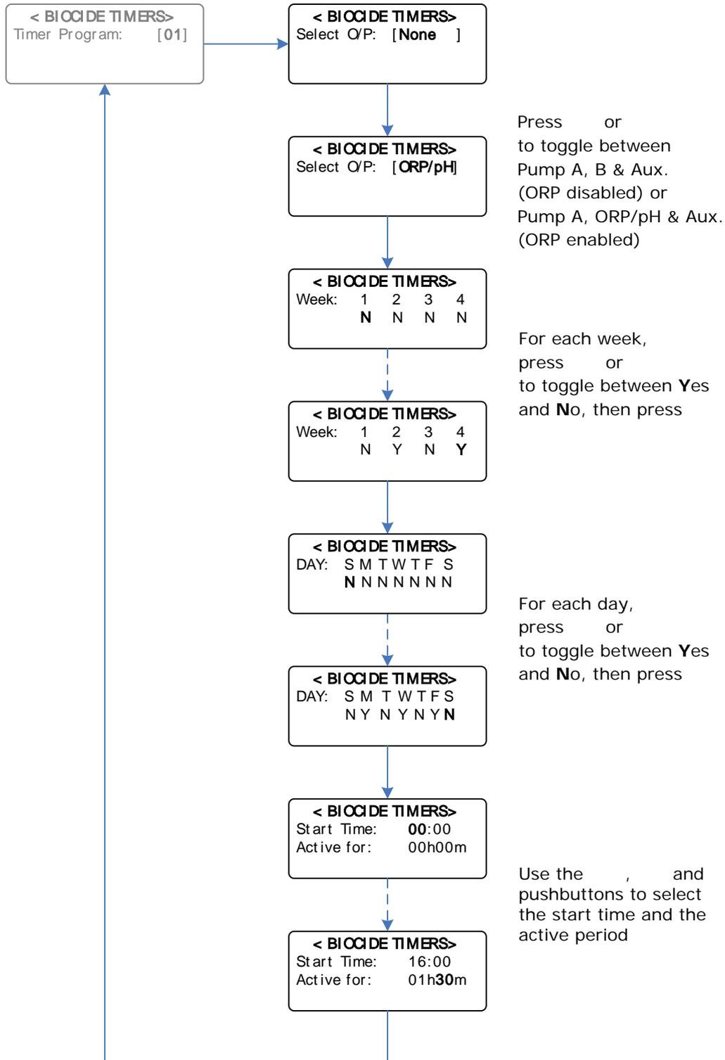
**Example:** Selecting Biocide Program 1, for the ORP & pH control functions to be active on Mon, Wed, Friday in Weeks 2 & 4, active for 1h30m, commencing at 16h00. Therefore the ORP & pH control only occur between 16h00 and 17h30 on the days selected.
