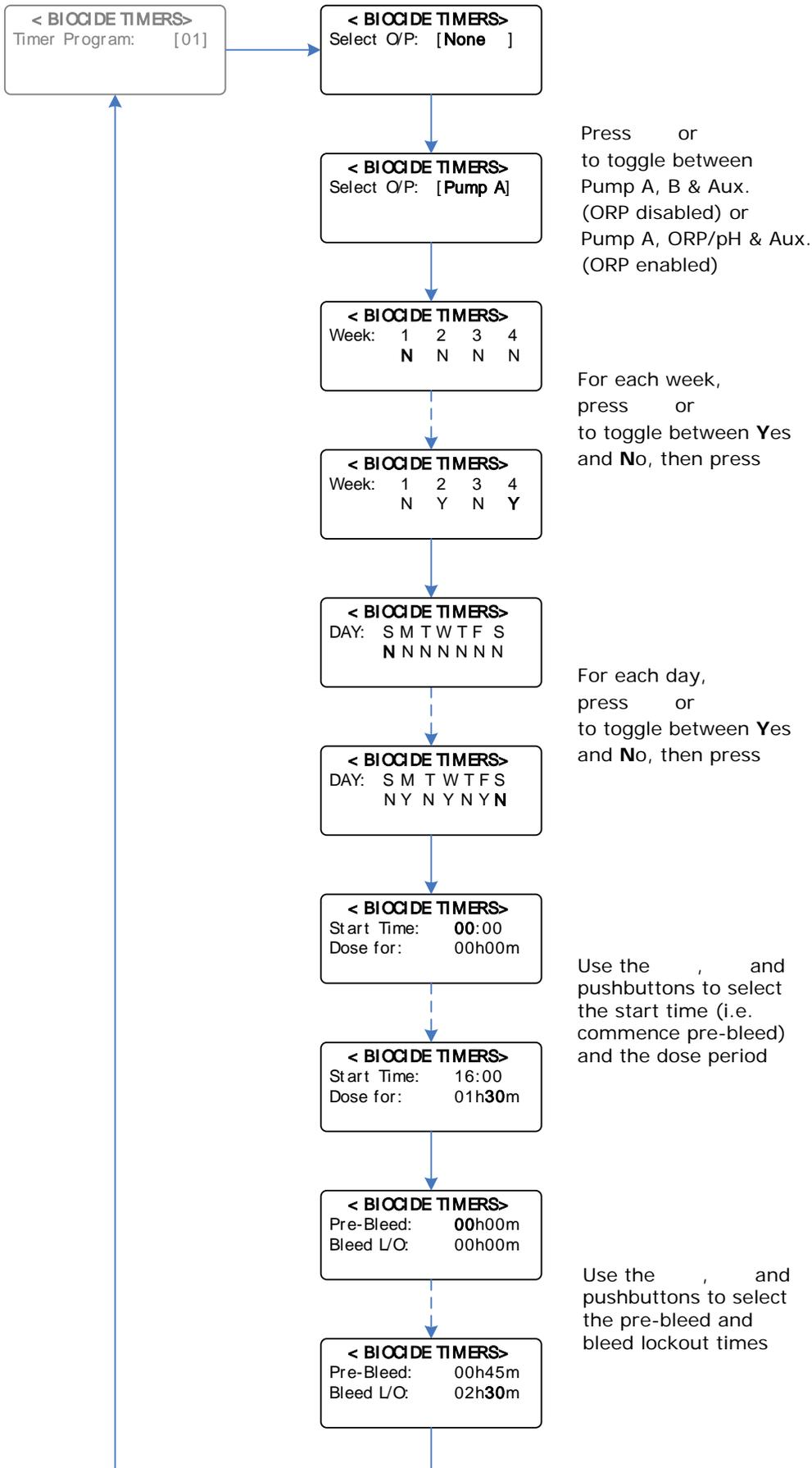
**Example:** Selecting Biocide Program 1, for pump A to dose on Mon, Wed, Friday in Weeks 2 & 4, with a 45m pre-bleed starting at 16h00, thereafter dosing for 1h30m, with an additional bleed lockout of 2h30m
