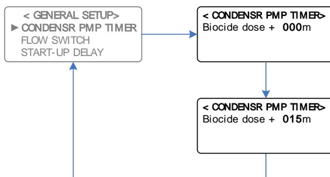
**Example:** Setting the Condenser Pump Timer for 15 minutes
