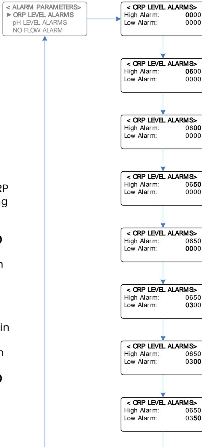
**Example:** Setting a High Alarm of 650mV and a Low Alarm of 350mV
