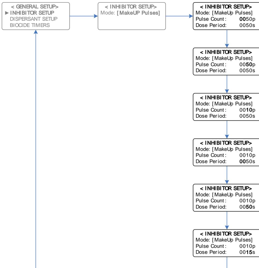
**Example:** With Inhibitor on “Make-Up Pulses” mode currently set – Setting the Inhibitor pump to dose for 15 seconds after 10 pulses from a water meter
