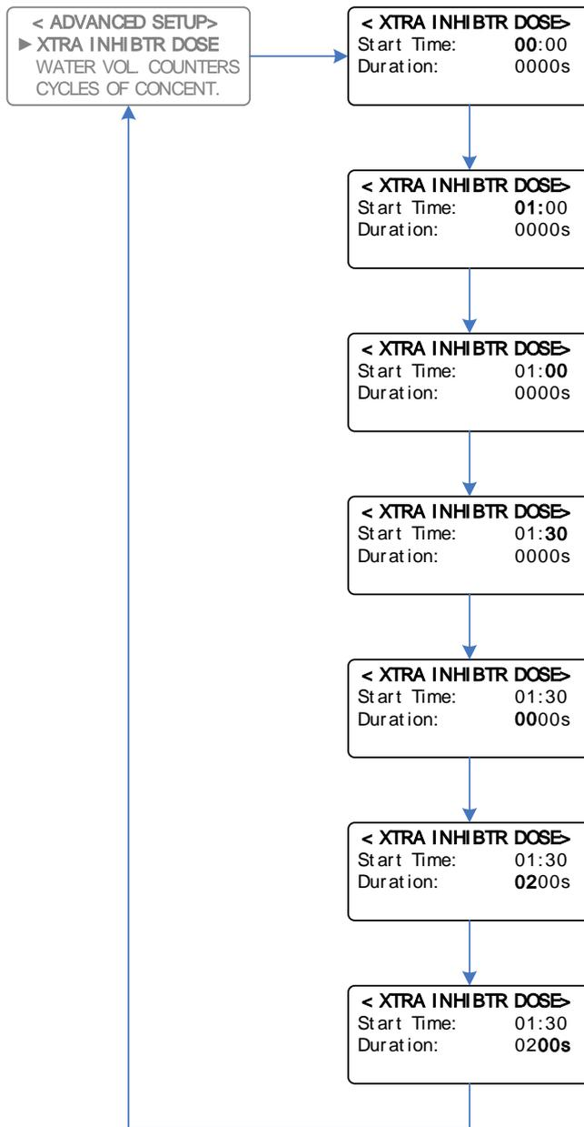
**Example:** Setting up an Extra Inhibitor dose, starting at 1:30, dosing for 200 seconds
