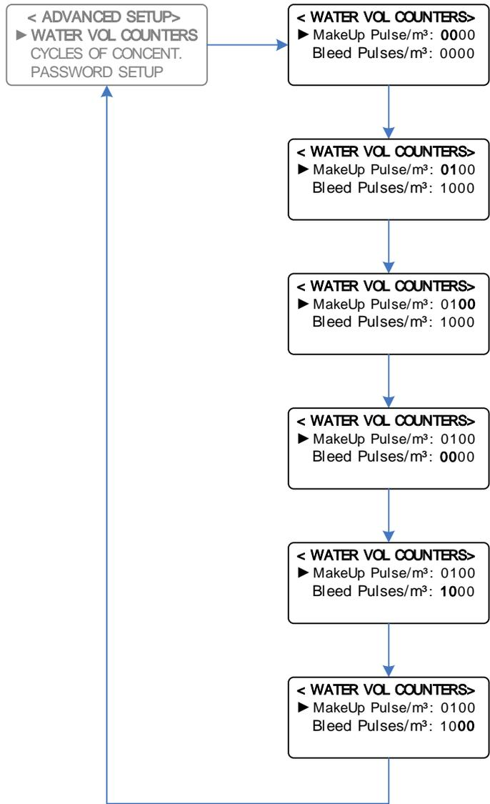
**Example:** Setting Make Up Pulses to 100 pulses / m<sup>3</sup> (1P/10L), and Bleed Pulses to 1000 pulses m<sup>3</sup> (1P/L)
