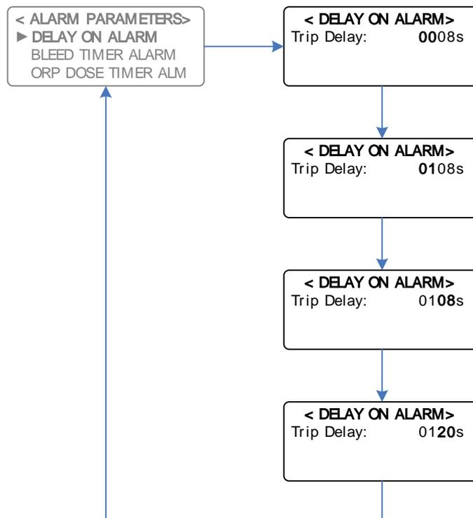
**Example:** Setting the Delay on Level Alarms to 2 minutes
