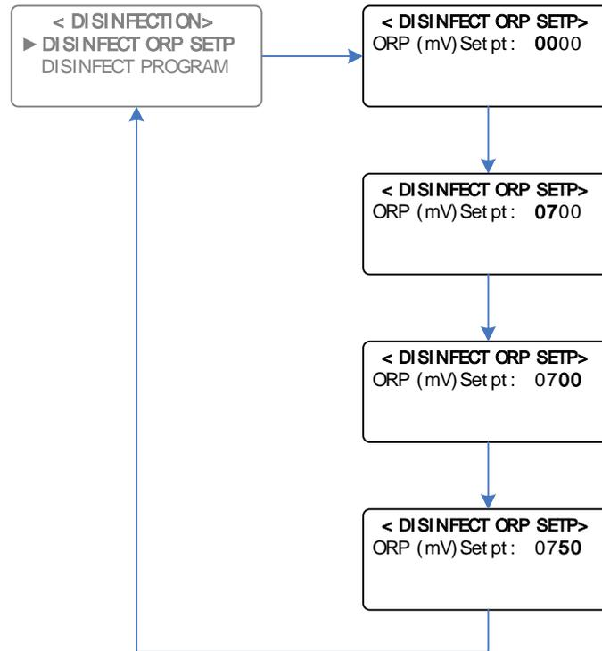
**Example:** Increasing the Disinfection ORP Setpoint from 500mV to 750mV
