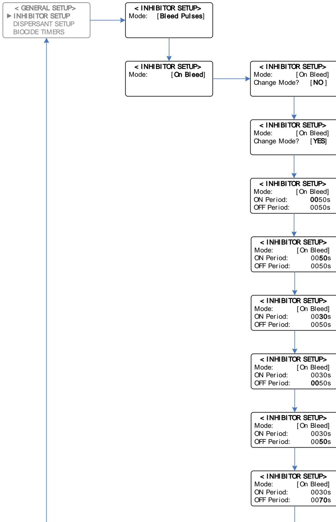
**Example:** Changing Inhibitor from “Bleed Pulses” mode to “On Bleed” mode -
