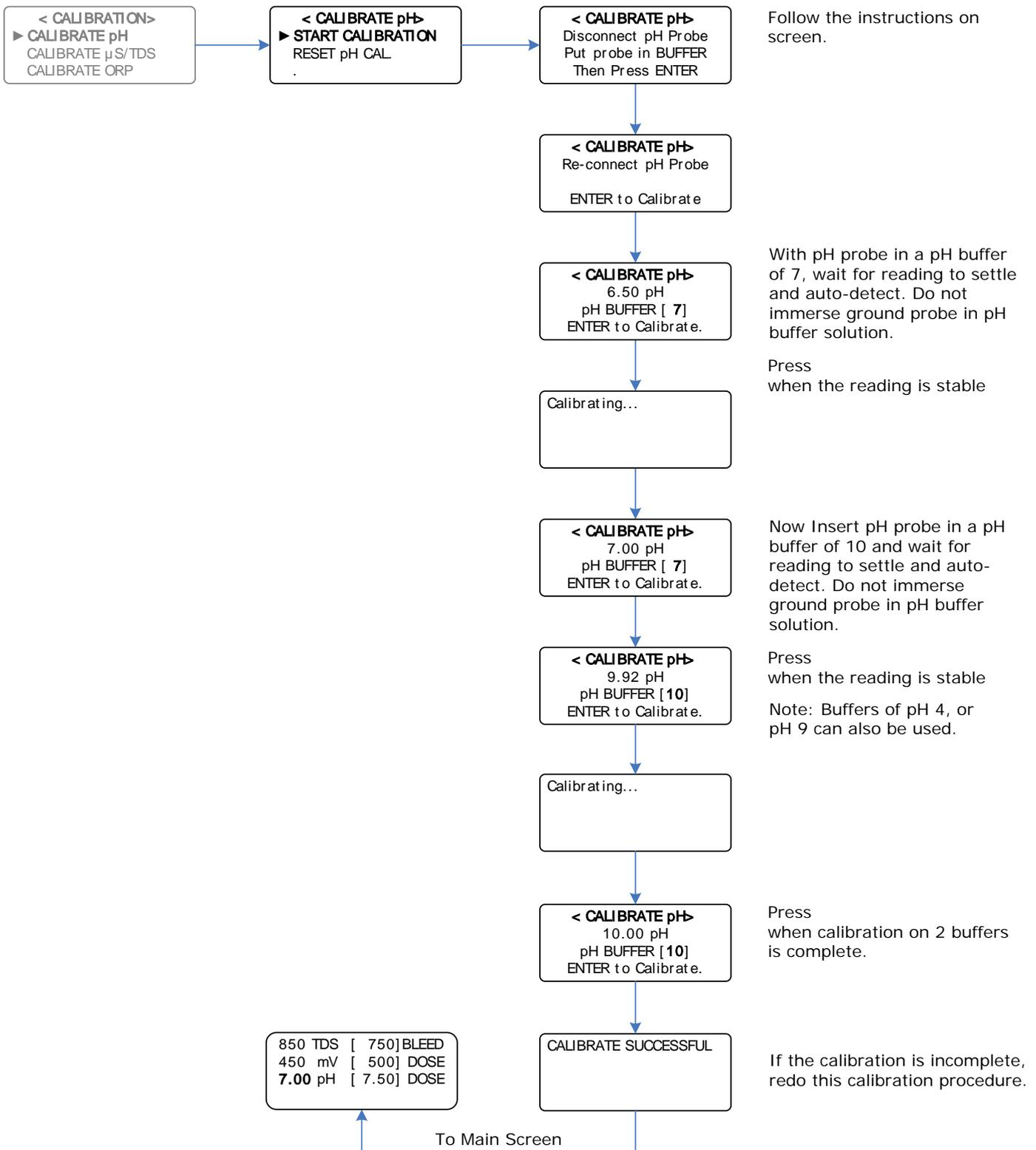
**Example:** Calibrating the pH for a reading of 6.5 pH in a 7 pH Buffer Solution, and a 9.92 pH reading in a pH Buffer Solution of 10 pH
