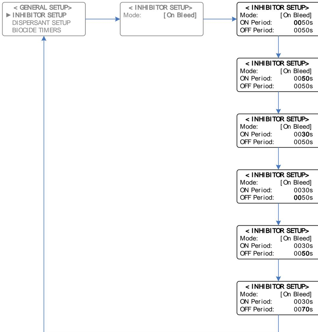
**Example:** With Inhibitor on Bleed mode currently set - Decreasing Inhibitor pump duty cycle from 50% to 30%
