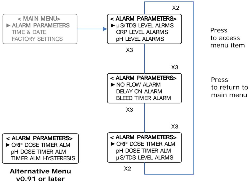
The controller has 8 programmable alarm functions as outlined above. If any of the alarms are activated and confirmed, the common alarm contact switches, and the Alarm message is displayed on the relevant position on the Main Menu of the LCD.
