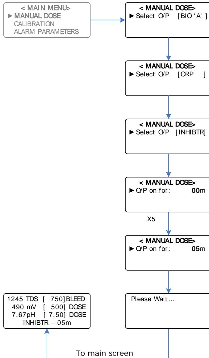
**Example:** Manual Dosing the Inhibitor for 5 minutes
