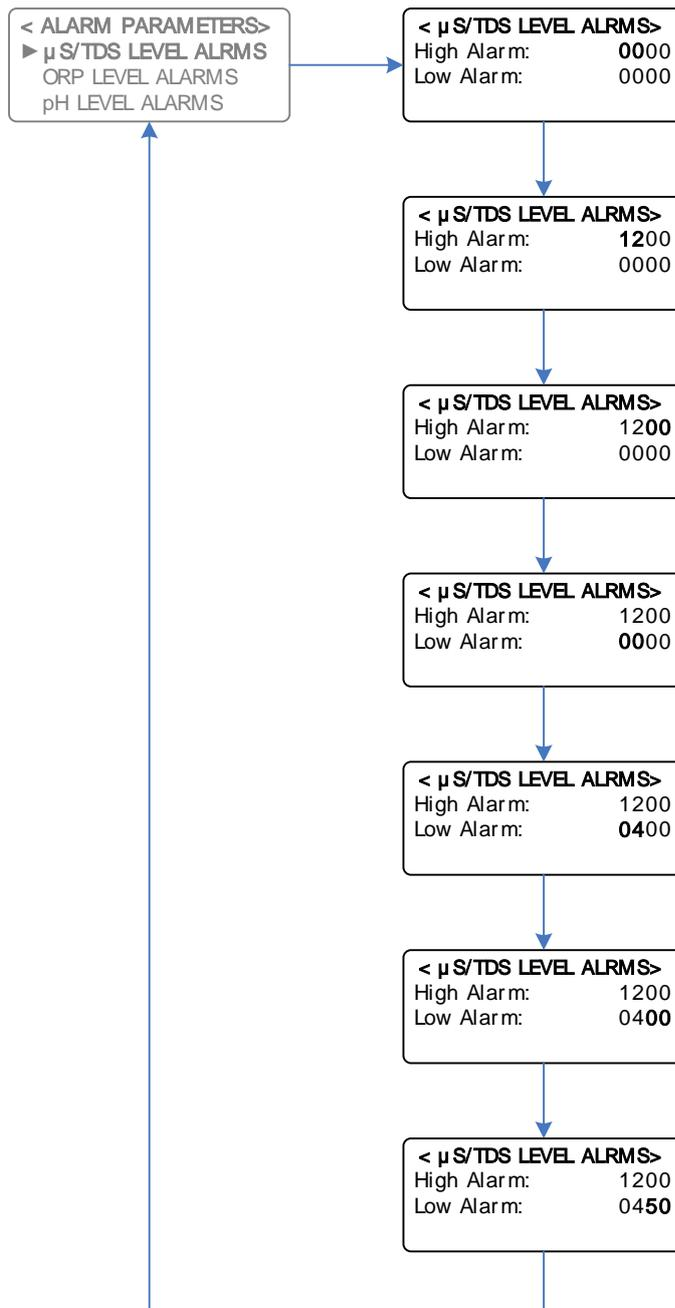
**Example:** Setting a High Alarm of 1200 TDS and a Low Alarm of 450 TDS
