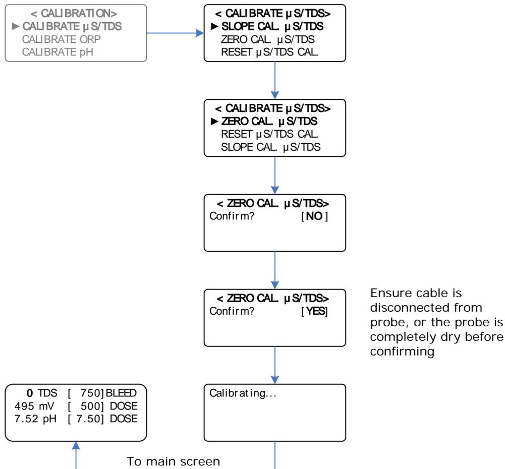
Calibrating the Zero for  $\mu\text{S}/\text{TDS}$
