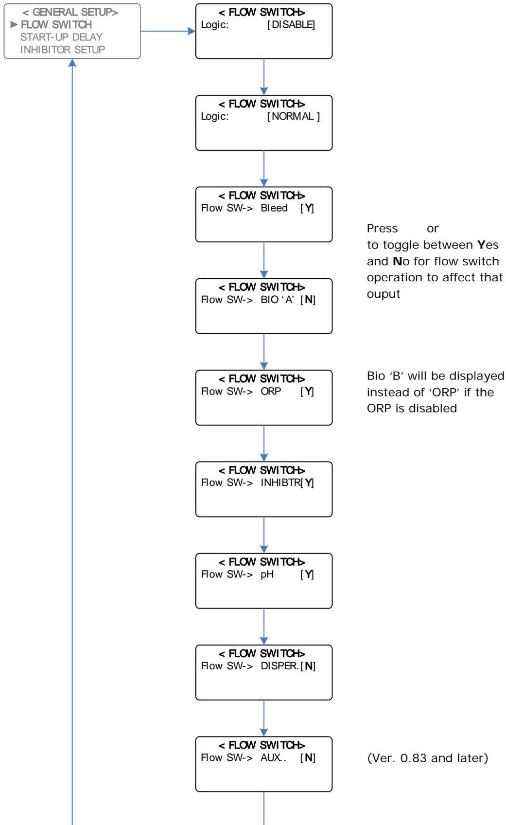
**Example:** Setting the Flow Switch to operate for Bleed, ORP, Inhibitor, and pH Functions
