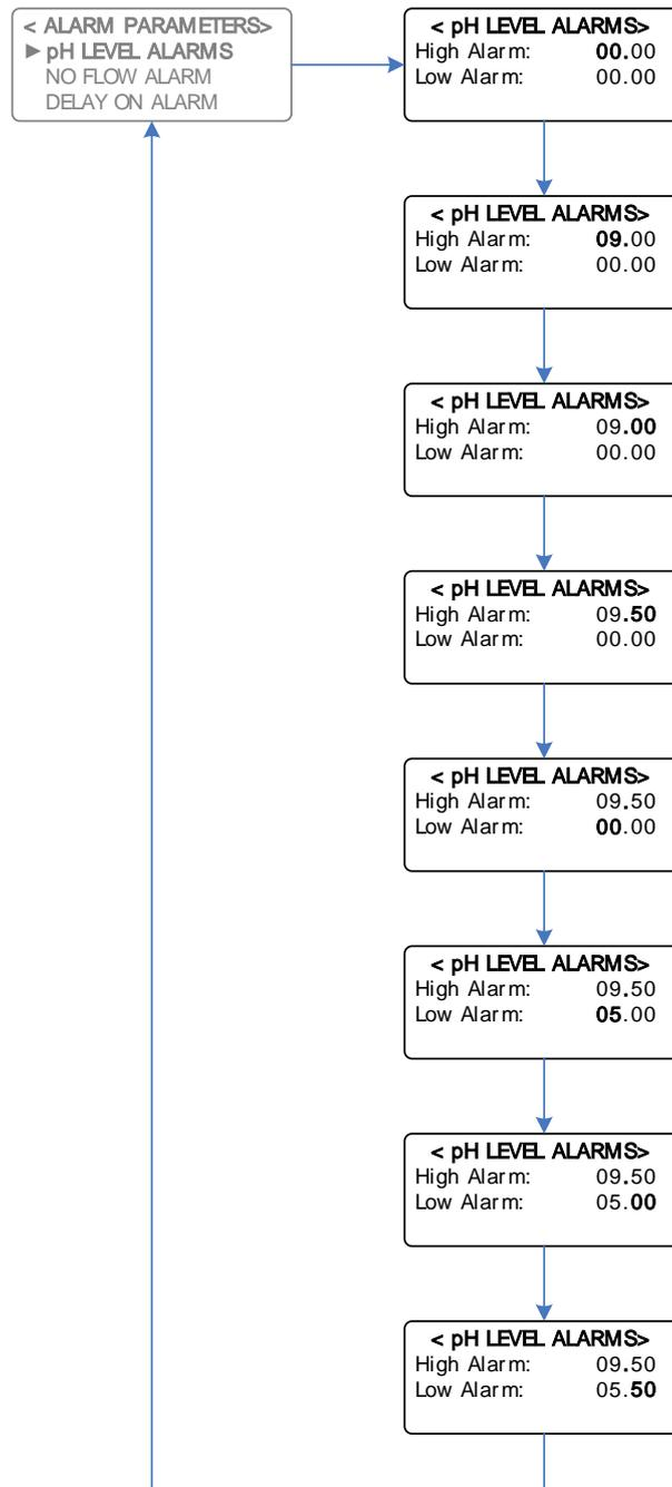
**Example:** Setting a High Alarm of 9.5 pH and a Low Alarm of 5.5 pH
