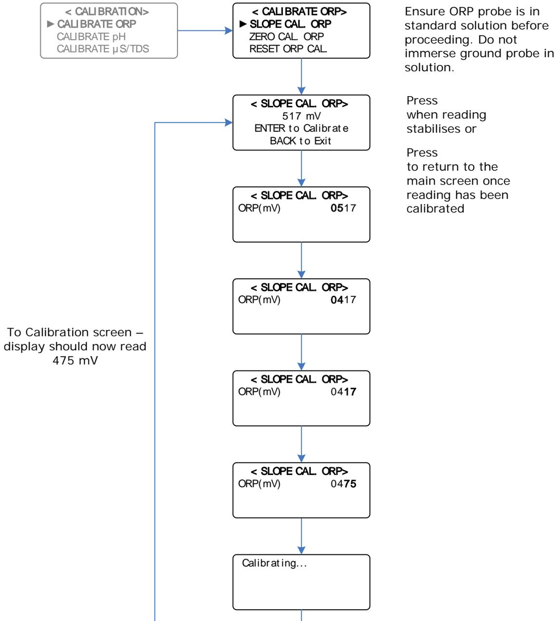
**Example:** Calibrating the ORP Slope Value from 517mV to 475mV
