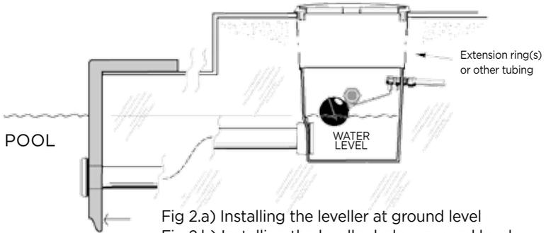
Fig 2.a) Installing the leveller at ground level
