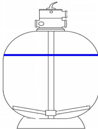
1. Check the filter size to determine the amount of media required. (see filter data table).
